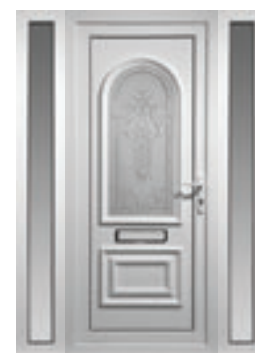
■ 1 x PVCu residential door set ■ 2 x narrow residential sidelites External frame dimension width = the door set width + 600mm External frame dimension height = 2055mm excluding cill
