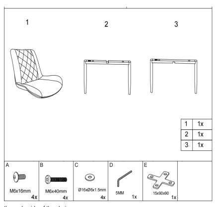
Handy Hint: insert bolts into the corresponding holes in the underside of the chairs do not fully tighten. Once all bolts are inserted go back round each bolt and then fully tighten.
