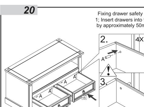
Fixing drawer safety stops 1; Insert drawers into frame by approximately 50mm.
