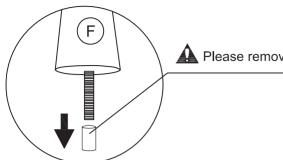
A Please remove the protective cap on the tip of thread before assembling.
